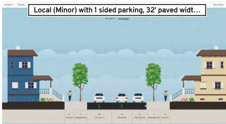
Figure 2 Example local (minor) street with 1 sided on-street parking, terrace, and sidewalks, 32' pavement width, 56' ROW
